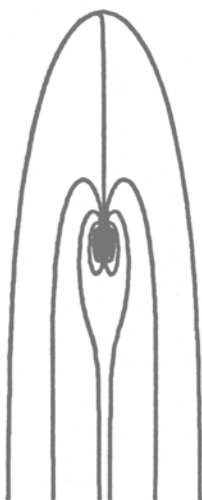
Figure 7.46 Phreatic surface and streamlines for \alpha = 90^\circ .
