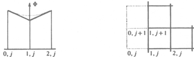
Figure 9.2 A boundary with \partial\Phi/\partial n given.
