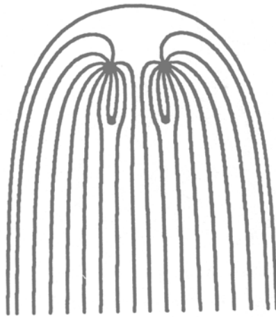
Figure 7.38 The flow domain with two recharge drains and two drains.
