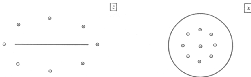
Figure 6.33 The distribution of poles in the z and \chi planes used to generate flow patterns in Figure 6.31 and Figure 6.32.
