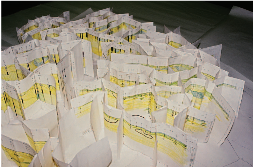
Figure 2. Paper sectional model for the NAGROM model of the northern part of the Netherlands.
